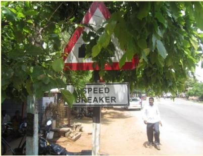
**CONSPICUOUS** – the sign must be able to be seen. This is a new and reflective sign but has been poorly located and it cannot be seen by drivers/riders. If a sign cannot be seen it cannot be of any use to the road users.
